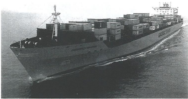
The Maersk pavilion explained the reliance of the world on the company's container ships exemplified by the 50,000 gross tonne British registered Greenwich Maersk . With a deadweight tonnage of over 62,000 tonnes she can carry 4,300 teu
